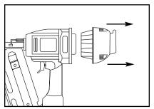
Figure 6. Removing nailer exhaust cap.
